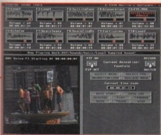
When GVP's IV-24 (or the upcoming OpalVision video module) is used, a PIP preview of the incoming animation can be displayed on DST's screen
